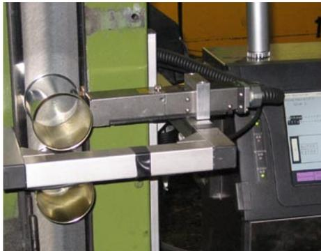
designed stainless steel cabinet, sealed to IP55 standards and capable of handling harsh industrial environments and deep cleaning regimes common in food process industries. Essential consumables are housed in the base of the cabinet.
